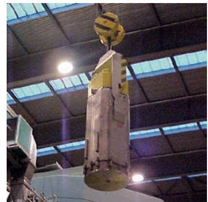
NEURAP transport/manipulation cask for highly radioactive samples.
