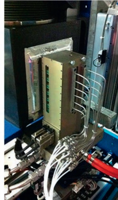
With the multicell setup, up to 6 small scale operating fuel cells can be imaged simultaneously P. Oberholzer et al., Electrochem. Commun. 20, 67 (2012)
