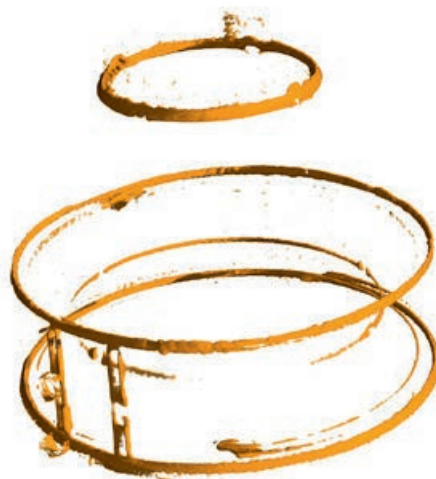
A non-invasive inspection tool for boron containing soldering connections is found in neutron imaging. A destructive inspection is not required when neutron tomography is applied to the object on the left. By suitable software tools the metal can be separated from the solder distribution show on the right. C. Grünzweig et al, 9th Int. Conf. Proc. on Brazing, High Temperature Brazing and Diffusion Bonding (2010)
