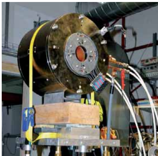
Fig. 3.4.1.1: Gun solenoid on his test bench (the steerers V and H are visible on front plane).
