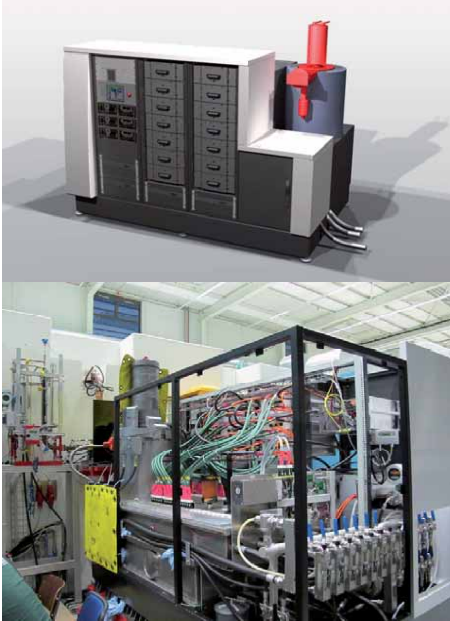
Fig. 3.2.4.4: Drawing of the high-power modulator K2 from the company SCANDINOVA (10–60MW; 200–450 kV) (top), and photograph of the installed prototype at the SwissFEL Injector Test Facility (bottom).
