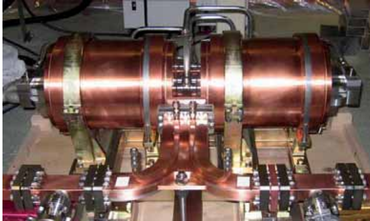
Fig. 3.2.3.4: SKIP pulse compressor used at KEK
