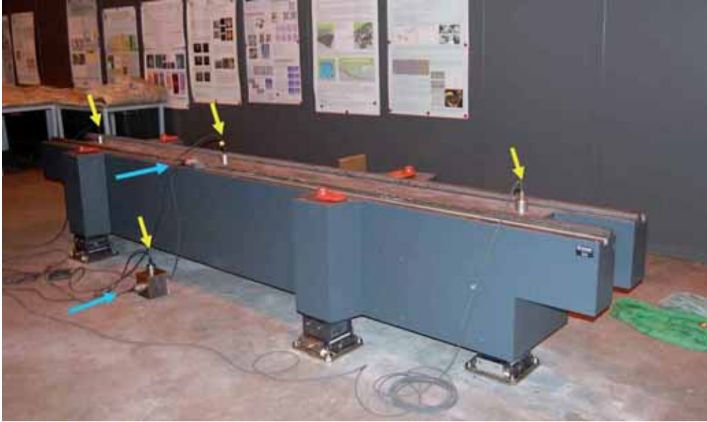
Fig. 3.8.3: Girder during eigenfrequency measurements: the arrows indicate the location of the accelerometers; test location at the SLS facility
