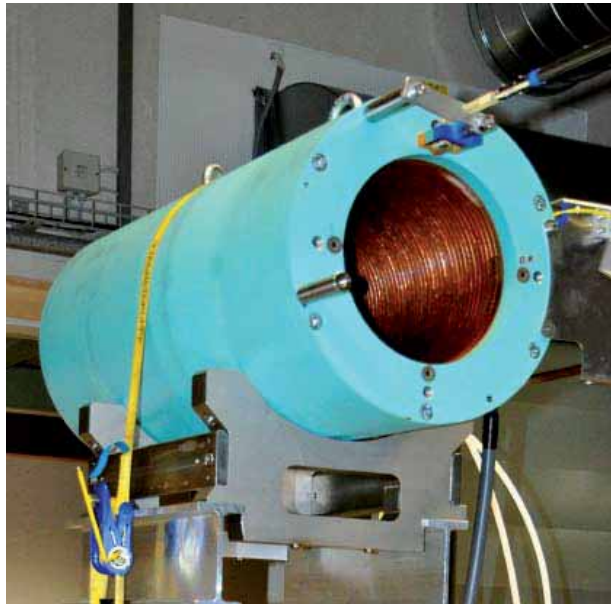
Fig. 3.4.1.2: S band solenoid on his test bench.
