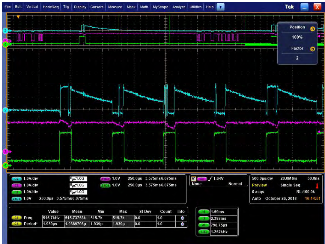
Figure 58: Example of a MSCB transmission measured with a oscilloscope. The blue line is the MSCB bus, the green line is an output enable signal for the used converter chip.
