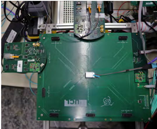
Figure 39: Picture of the clock distribution board.
