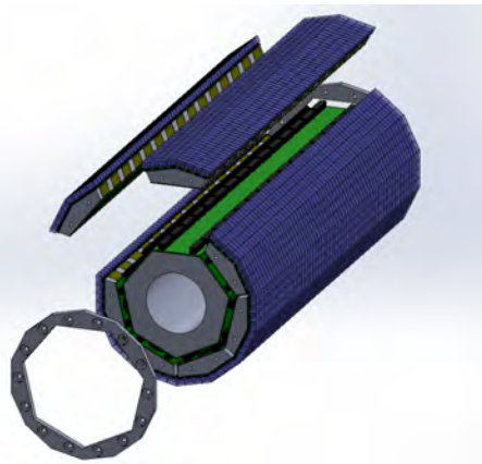
Figure 16: CAD drawing of a Mu3e recurl station with tile detector modules
