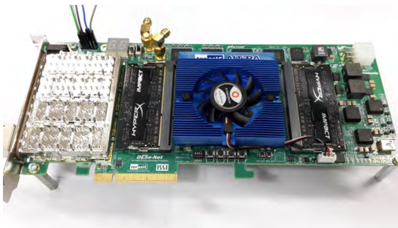
Figure 32: Picture of the DE5a-Net development board, which is used as optical receiver inside of each farm PC in the Mu3e DAQ.
