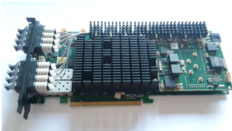
Figure 31: Picture of the PCIe40 board developed by the LHCb collaboration.
