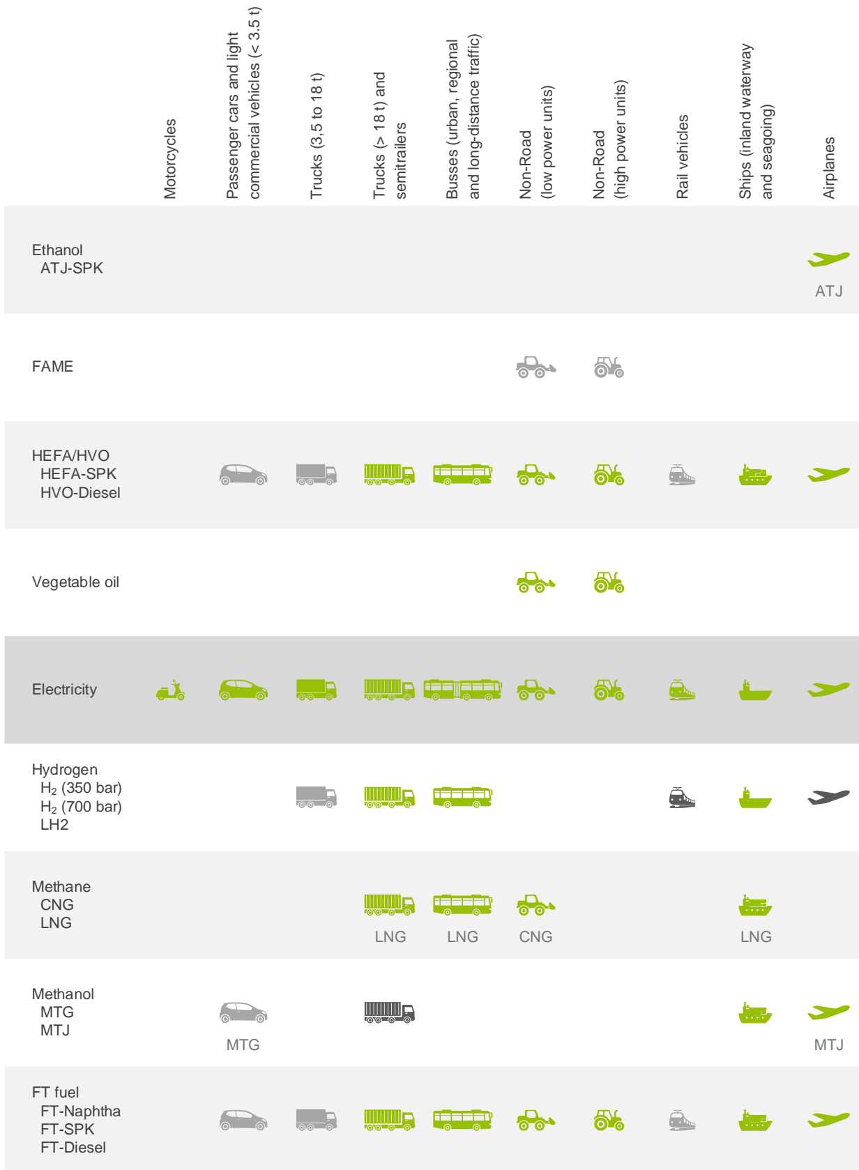
Figure 9-3 Vehicle-energy-matrix for 2045 (green – very probable option, black – possible option, light gray – option for remaining stock)
