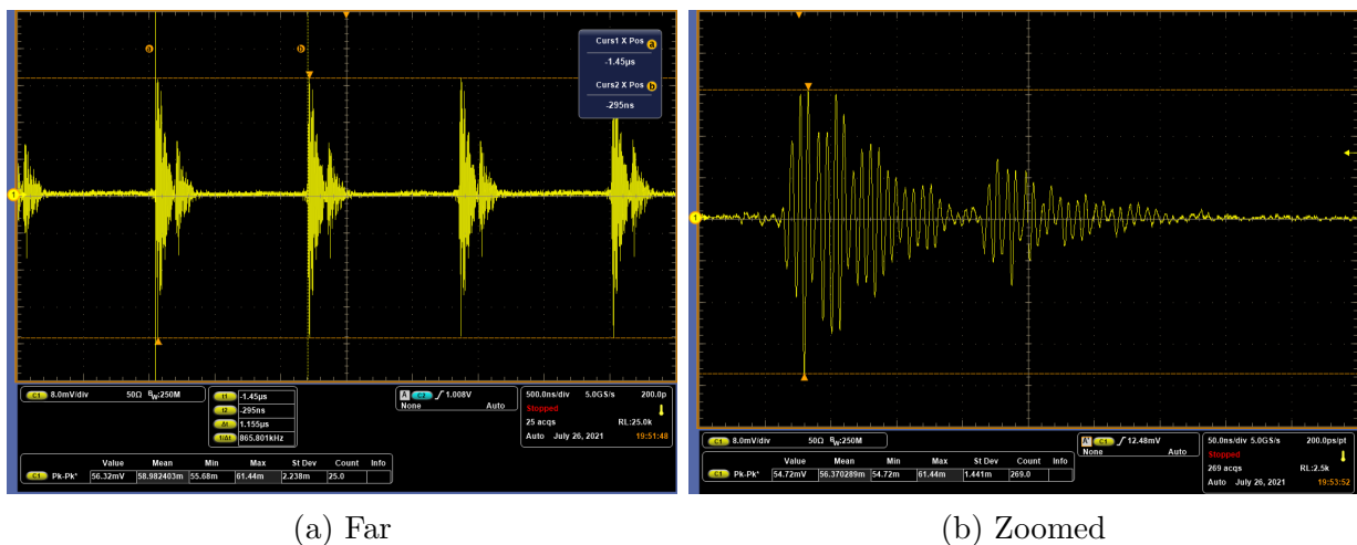
Figure 5.10: HF noise with peak-to-peak voltage approx. 60 mV (250 MHz bandwidth).
