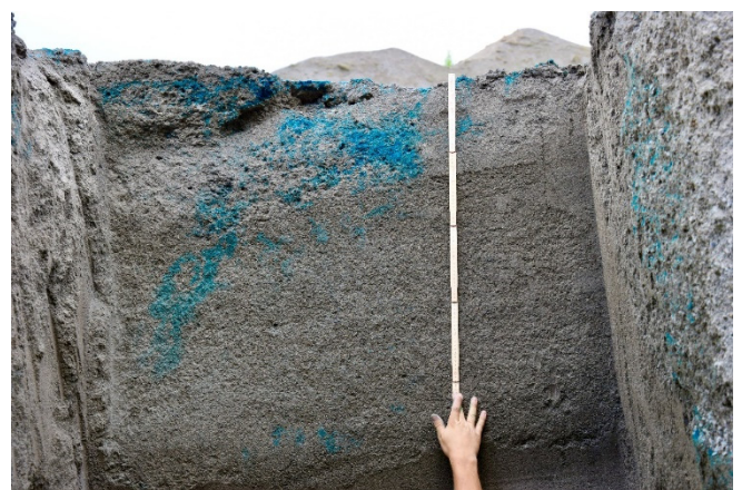
Fig. 8.5: Lateral view of the excavated experimental site. The used dye tracer Brilliant Blue visualized the occurring preferential flow paths through the bottom ash landfill body.
