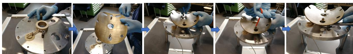
Figure 3: fixing the spring loaded mu-metal liner into the microjet flange
