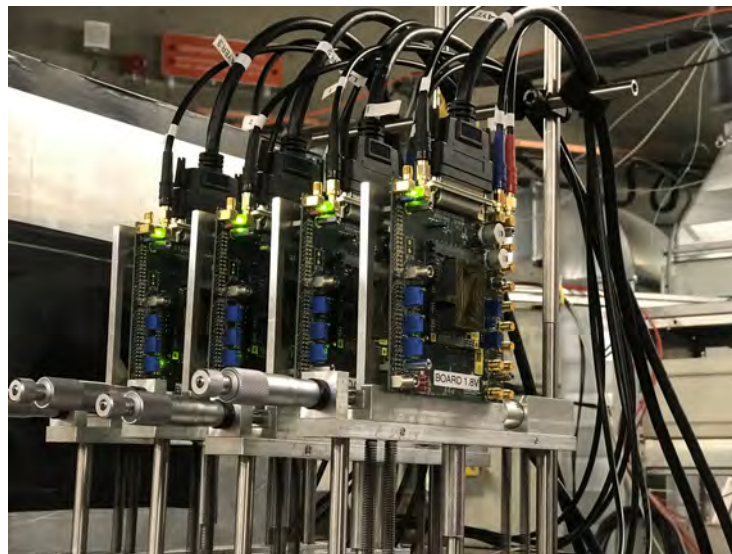
FIGURE 10.2: Picture of the MuPix8 Telescope layout. Four sensors are mounted on PCB boards.
