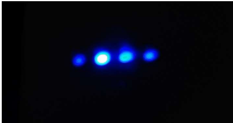
Figure 4.4: Picture of a diffraction pattern of double-passed light on a piece of paper. The brightest spot is from +1 order diffraction. To right of it, we have 0th and -1 order diffraction, and to the left, +2 order. When you see a diffraction similar to this with a piece of paper, you can be more or less confident that you indeed have the maximized first order coming out of the AOM.
