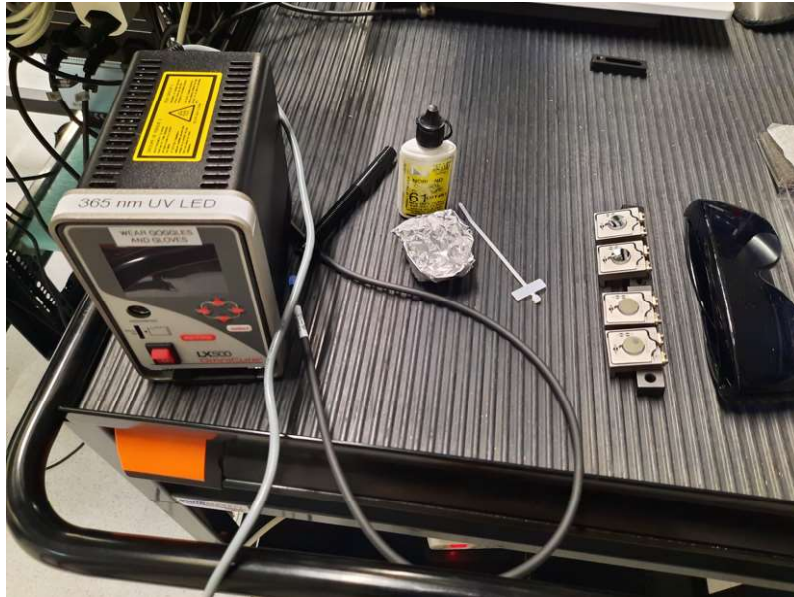
Figure A.2: Picture of the optics glue-in setup. The UV-curing light controller shown on the left is connected to a LED pen which outputs the curing light and a foot pedal (not shown in the picture) which one can press down to turn on the light.
