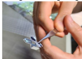
cutting of reflective foil
