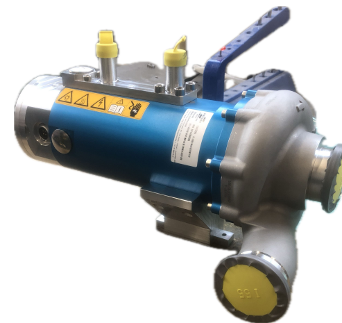
Turbo compressor providing 16 g/s helium (from FISCHER spindle)
