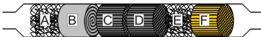
Figure 3-1: Scheme of the reactor for the pulsation-free formation of water vapor by the reaction of \text{H}_2 with \text{O}_2 in \text{N}_2 . (A, E) glass wool, (B) flame arrester, (C, D) catalyst-coated monoliths and (F) uncoated cordierite monolith to retain the glass wool.
