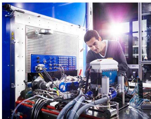
Fuel cell system testing. Experimental set-up for advanced start/stop investigation.
