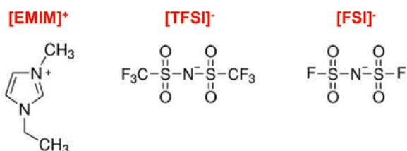
Scheme 1: Ionic species comprising the ionic liquid electrolytes employed for electrochemical graphite cycling.
