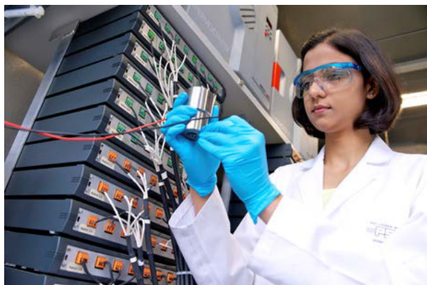
Multi-channel battery testing facilities.
