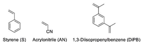
Figure 1: Monomers used for the preparation of radiation grafted membranes.
