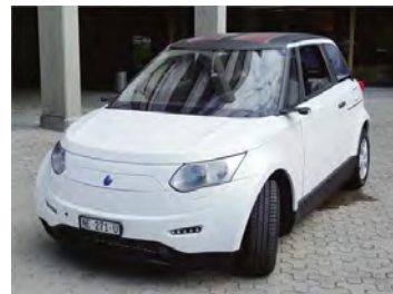
Figure 3. Belenos-PSI vehicle for fuel cell system tests.
