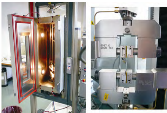
Figure 1. Zwick Roell tensile testing machine and attached climatic chamber (left) and Vulkollan coated sample holder (right).
