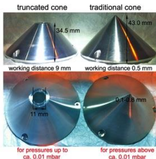
Fig. 2.6. Entrance cones of the Scienta HiPP-2 R4000 electron spectrometer used with the liquid microjet. The truncated cone exposes the L1p element to the measurement zone and allows for an accelerating field to be applied to photoelectrons below 60 eV. The working distance of the truncated cone is 9 mm. The traditional cone is used in liquid microjet studies at ambient pressure conditions up to 20 mbar and has an aperture diameter typically between 0.1 and 0.8 mm. The working distance of the traditional cone is on the order of the aperture diameter.
