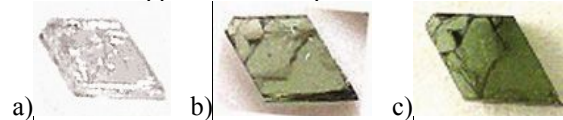
Fig. 1: Natural diamond sample n3C22: a) before irradiation; b) after a epithermal neutron dose of 4.3 \times 10^{14} \text{n}/\text{cm}^2 ; c) after an additional dose of 3.8 \times 10^{14} \text{n}/\text{cm}^2 .
