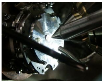
Fig. 1: Cu sample holder with ice, HCl dosing tube, and electron sampling aperture.
