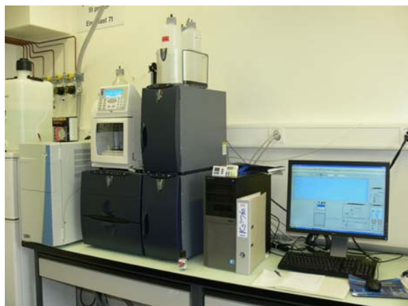
Fig. 5.3: HPIEC-MS equipment (left) and chromatogramme for acetic acid and oxalic acid (right). The HPIEC systems consists of a IonPac AS11-HC column (Dionex, Sunnyvale, CA, USA), a GP 50 gradient pump, an EG 40 eluent generator, an AS 50 auto-sampler coupled to a CD 25 conductivity detector, and a MSQ™ Plus (Thermo Fisher, Sunnyvale, CA, USA) MS electrospray (ESI) operated in the negative ionization mode
