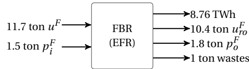
FIGURE 3.4: Inputs and outputs of the FBR
