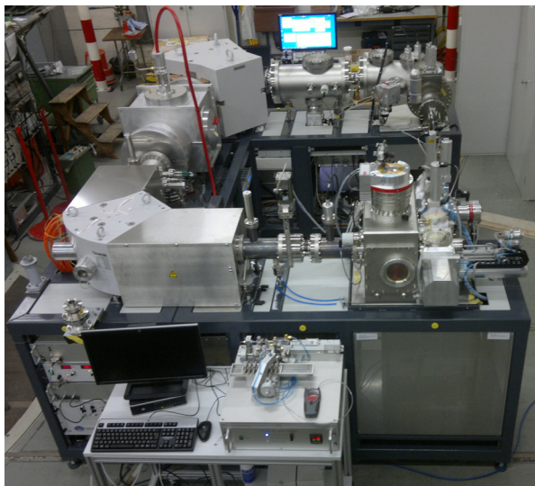
Fig. 1: The new MICADAS during the testing phase with the gas inlet system at the front.
