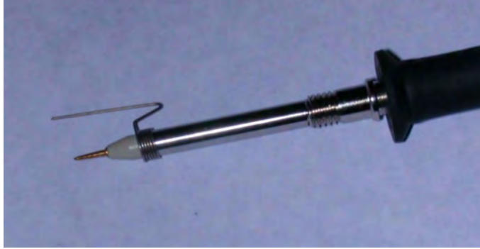
Figure 3.3: Pigtail probe for the oscilloscope for a proper measurement. The short distance of the non coaxial circuit reduces the pickup noise [12].
