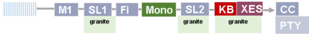
Figure 11.9: Different packages for the beamline upgrade in relation to the beamline elements. Different colors represent different work packages. Grey: unchanged elements, light green: package ‘maintain and coherence’, green: replaced monochromator, red: added Johansson emission spectrometer. Upgrade of KB system (KB) and new endstation (XES) are not completely independent, as both elements are located on the same granite block, and use interconnected vacuum chambers. M1: first mirror, SL1: slit at intermediate focus, Fi: filter for high harmonics suppression, SLS: entry slit for KB system, CC: existing mobile chemistry chamber, which is also operated at PHOENIX II, PTY: potential mobile high resolution ptychography endstation
