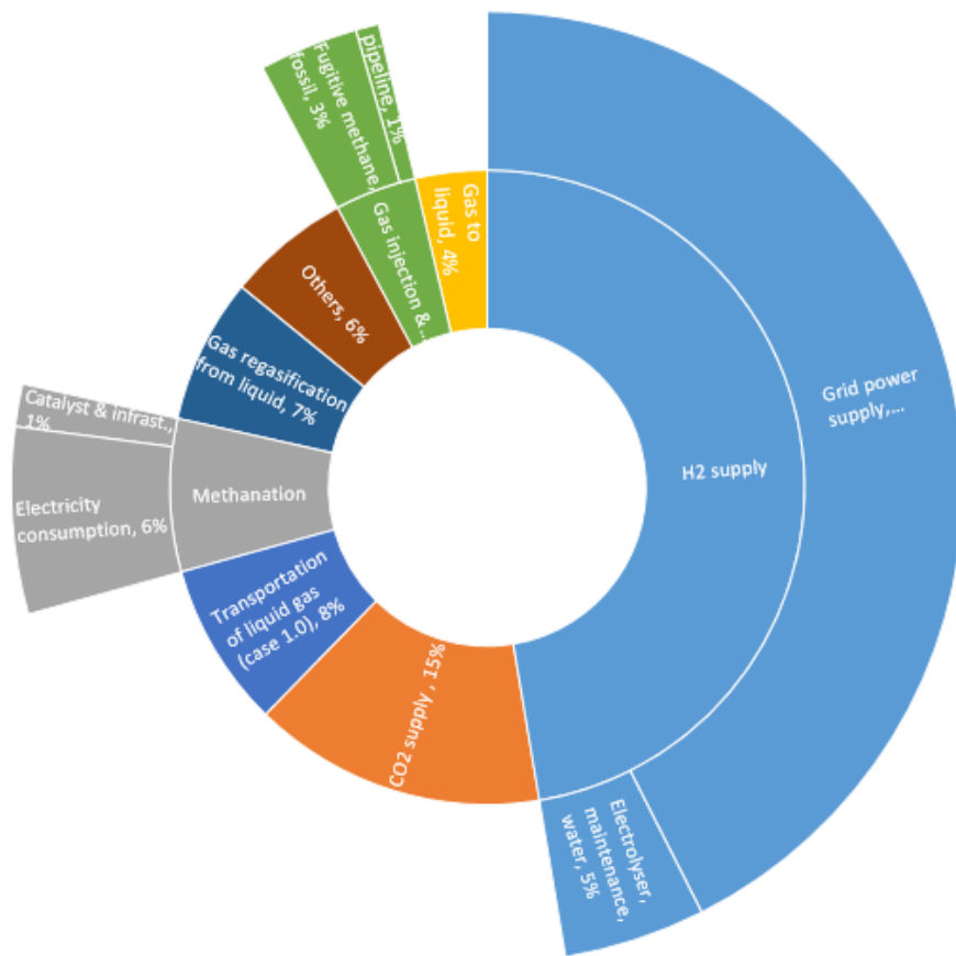
Figure S4 Contribution analysis of life cycle GHG emissions of SNG production and supply (transport case 1.0); 100% Icelandic grid supply for electrolysis; “Others” include other processing facilities throughout the production and supply chain (e.g., condensation unit after methanation, etc.).
