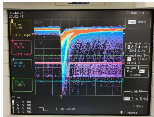
Figure 7.77: An example of the Pill signal at the oscilloscope. The high amplitude waveforms are associated with the muons while the low ones with the positrons (in this case cut by the trigger threshold). The separation between the two particle types is very clear.
