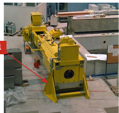
Figure 18.5: SINQ exchange flask when it was assembled: No 1 points to the turning support.
