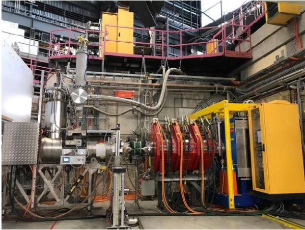
Figure 7.76: The pill detector mounted along the piE5 beamline. The scanner system is also visible.
