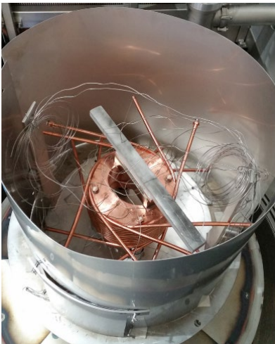
Figure 8.24: Mockup collimator in the vacuum oven after brazing.
