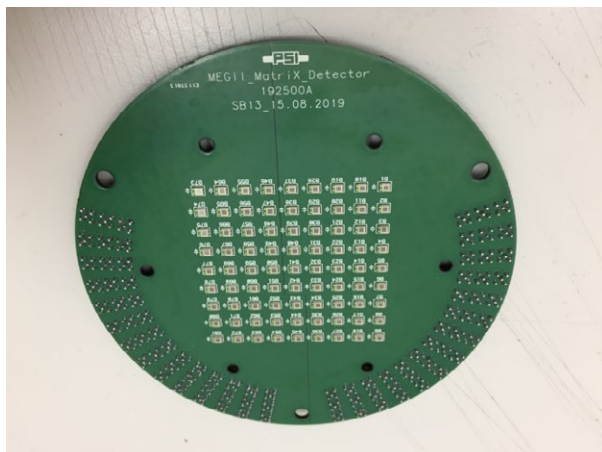
Figure 7.82: A picture of the Matrix detector prototype during the assembly stage. The MPPC matrix is on the left and BC400 scintillators are on the right.
