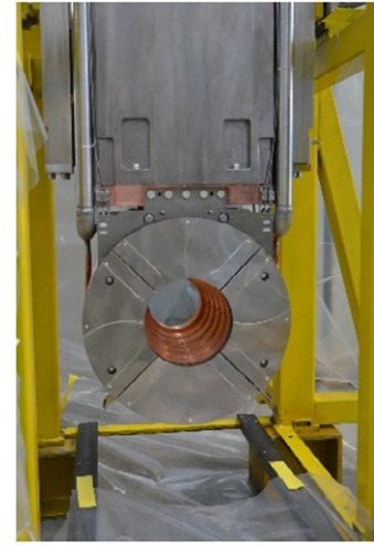
Figure 8.20: Beam Dump 1, assembling of the aperture.
