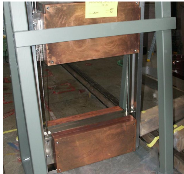
Figure 7.75: Picture showing one of the beam blockers used in the secondary beamlines of PSI during its construction. It is constructed as a sandwich of 90 mm copper, 120 mm stainless steel and another 90 mm copper.
