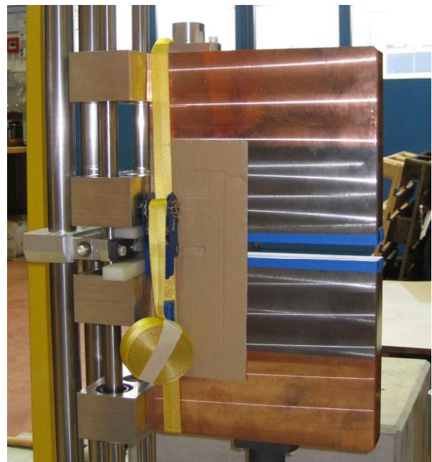
Figure 7.74: Photograph showing one of the slit systems used in the secondary beamlines of PSI during construction.
