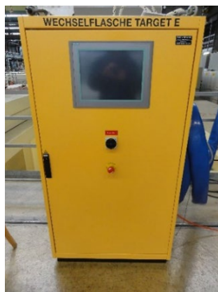
Figure 9.38: Control unit of the exchange flask.
