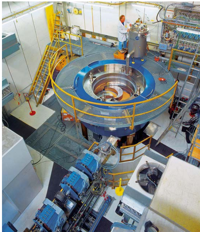
Figure 2.8.: Proton therapy treatments at PSI use an in-house built superconductor accelerator, a compact cyclotron, called COMET. It was especially developed for medical applications by the company ACCEL (now part of Varian Medical Systems) and brought into service in 2007. It delivers a beam energy of 250 MeV, which can be reduced when needed for patient treatments (see https://www.psi.ch/protontherapy/center-for-proton-therapy-cpt ).
