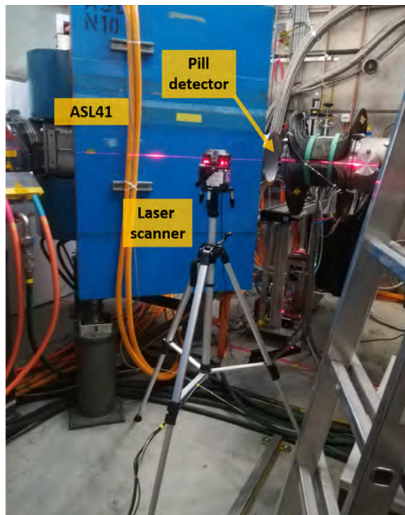
Figure 7.7: Alignment of the Pill detector for beam measurement at the collimator.
