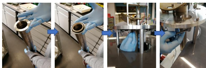
Figure 8: assembling the aluminum liquid catcher into the microjet flange
