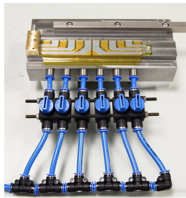
Chip alignment and ladder production tool for the vertex detector
