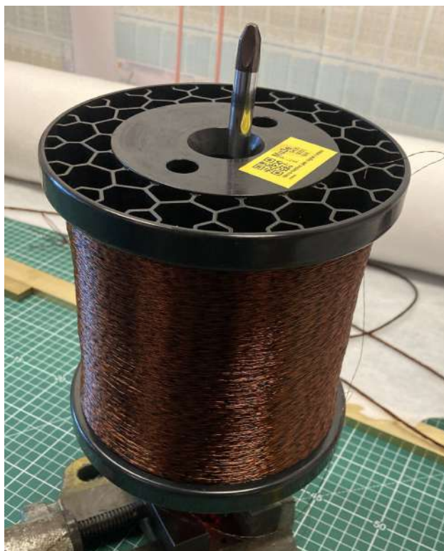
Figure 3.1: A coil for the raw micro twisted cable used for the Mu3e experiment.
