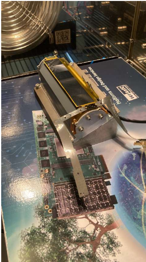
Figure 4.1: The ladder is screwed on the assembly tool and directly connected to the Endpiece Flex in the Climate Chamber.
