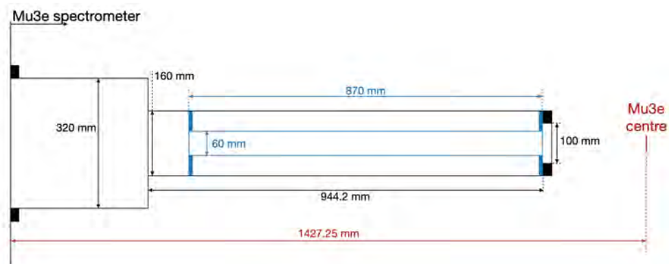
Figure 3.20: Sketch of the beam pipe and of the insert used for the commissioning at Mu3e center. The beam pipe has a diameter of 160 mm and an exit window with a diameter of 100 mm. The insert has a diameter of 60 mm.
