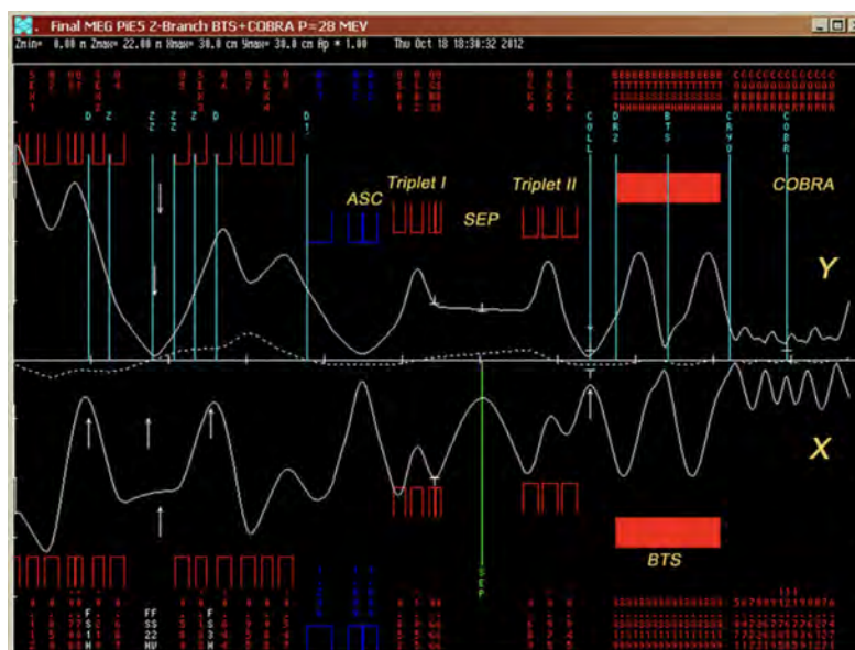
Figure 3.8: Second order envelope of the surface muon beam along the \pi E5 beamline in the MEG II configuration computed with TRANSPORT from [31]. Top: vertical envelope. Bottom: horizontal envelope. The dashed line represents the dispersion along the beamline in case of a momentum higher than nominal by 1%
