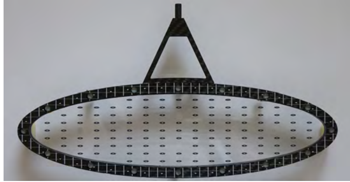
Figure 1.7: The MEG II target from [2]. A pattern of white dots on black background is printed on the scintillating foil and on the frame to monitor the position and possible deformation of the target through data taking.
