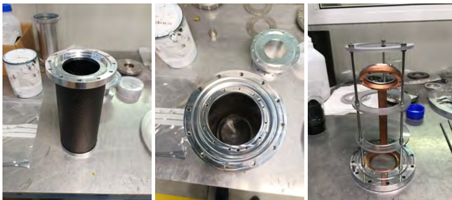
Figure 4.6: Left: carbon fiber vacuum chamber. The carbon fiber cylinder is glued to an aluminum endcap and to an aluminum flange. Center: carbon fiber vacuum chamber, inside. Right: target insert. The copper arm is bolted to an aluminum ring which fits into the flange of the chamber. Three stainless steel rods hold acrylic rings to reinforce the structure of the vacuum chamber. The copper target is secured on the arm with a ring to connect to the copper support with screws.
