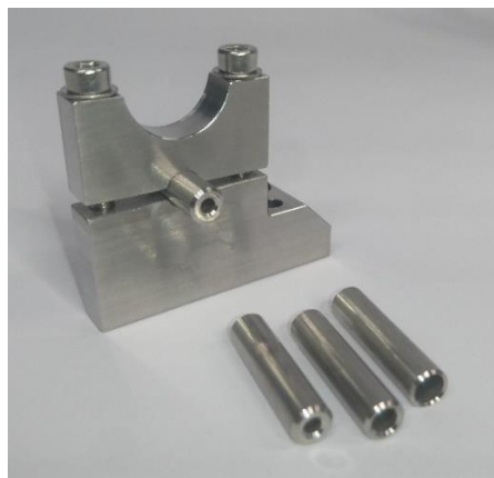
Figure 8: Types of steel pipes incl. mount
