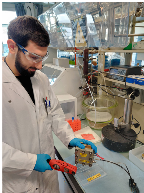
Master student Masis Sirim is assembling a proton exchange membrane fuel cell.
