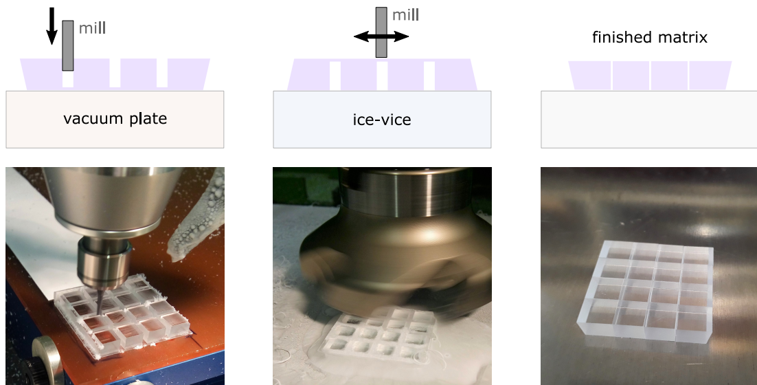
(a) Scintillator milling on the vacuum plate.
