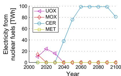
FIGURE 6.13: Enhanced nuclear cycle: Swiss electricity from nuclear fuels in noLWR scenario
