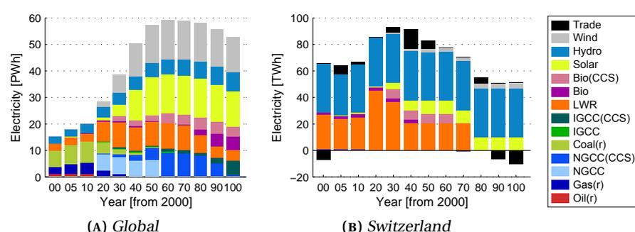
FIGURE 4.25: Reference stabilization scenario: Electricity production
