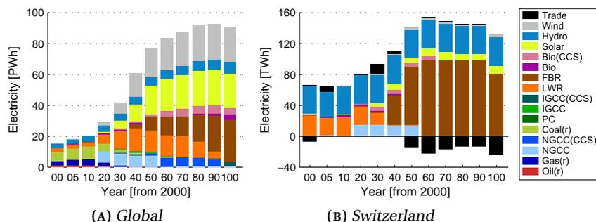
FIGURE 6.12: Enhanced nuclear cycle: Electricity production in no LWR in Switzerland scenario
