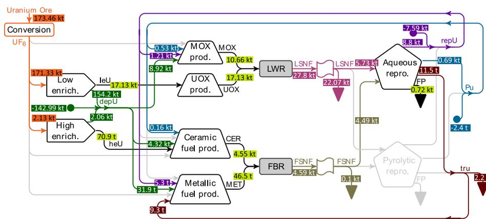
FIGURE 6.8: Enhanced nuclear cycle: 2040 global fuel flows in climate scenario with 100% nuclear support
