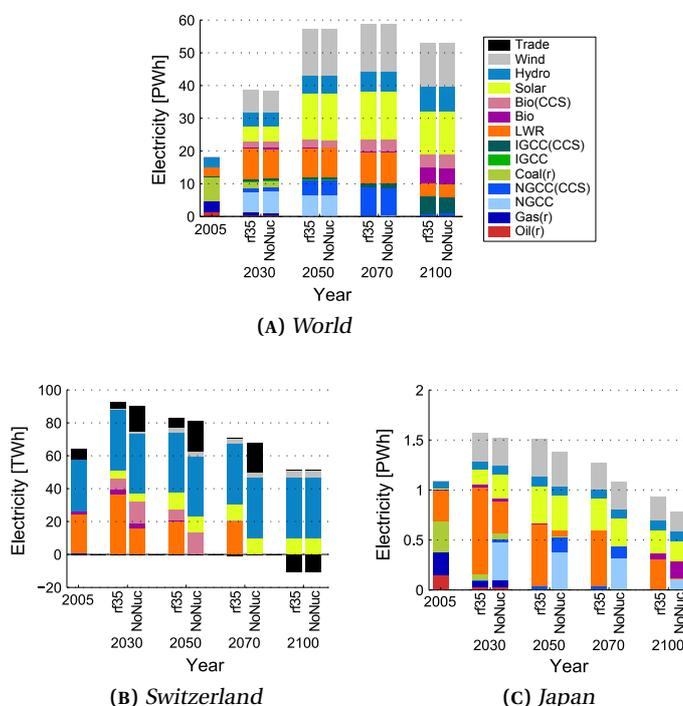
FIGURE 5.21: Nuclear phase-out in Switzerland and Japan: Electricity generation
