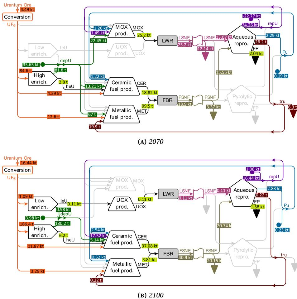
FIGURE C.1: Enhanced nuclear cycle: Fuel flows in rf35NC scenario
