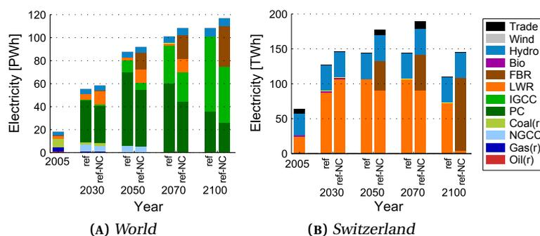
FIGURE 6.2: Enhanced nuclear cycle: Electricity generation in reference scenario
