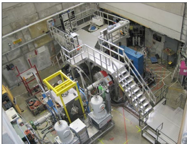
Figure 3: DOLLY instrument permanently installed in the \pi\text{E1} area. The spin rotator is visible in the bottom left part of the picture. The large platform allows easy access to the cryostats and for changing samples.
