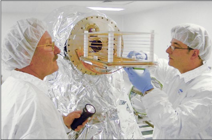
Figure 3: Assembly of the time projection chamber developed by the PSI Detector Group.
