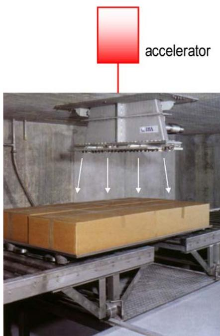
**Figure 2-2.** Electron-beam irradiation of goods conveyed under the scan-horn of an electron accelerator. Typical electron energy is in the MeV range (photo: Leoni Studer AG, Däniken SO, Switzerland).
