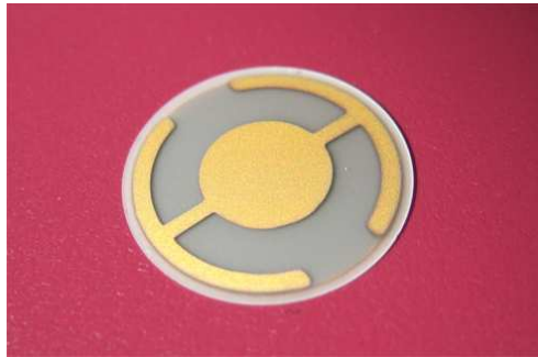
Figure 2.12: Resonator used in our quartz crystal microbalance.
