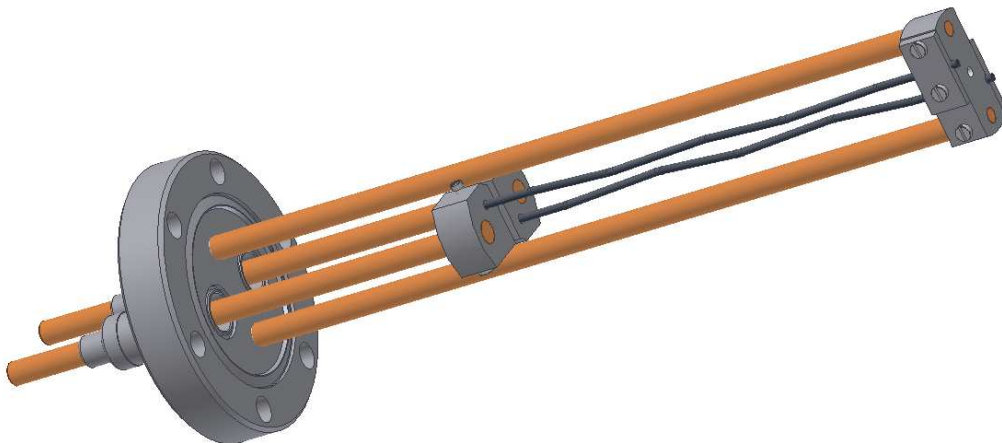
Figure 3.2: In-house built titanium sublimation pump.
