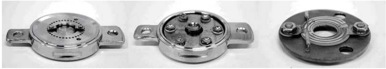
Figure 3.6: Picture of the sample holder. Left: top view, center: bottom view, right: inside view with the thermocouple and the heating element on an insulating Macor ® washer.
