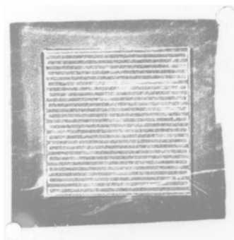
Figure 4: The pressure distribution in the experimental cell (active area 30 \text{ cm}^2 ). Dark colors indicate high pressure, bright areas low pressure.
