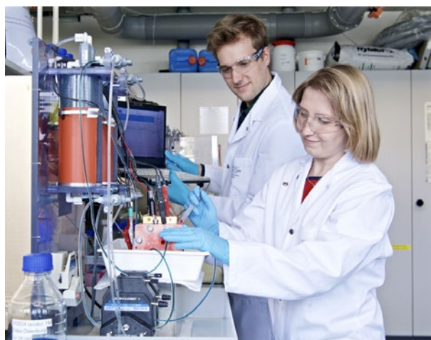
Device level characterization of an all-vanadium redox flow cell with a membrane developed in-house.
