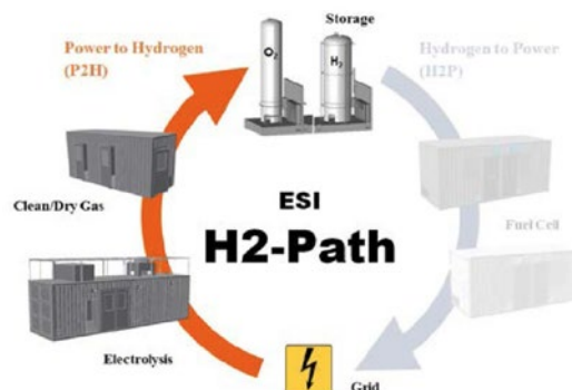
Figure 2. Schematic of the power to hydrogen process (P2H), consisting of a 100 kW Siemens PEM electrolyzer. Excess energy in the grid can be sunk and stored in the form of gas.
