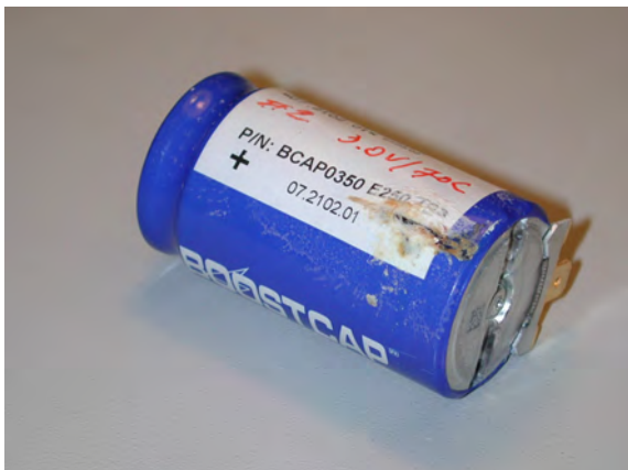
Figure 3. Picture of the opened can of a BCAP350 capacitor after the test at 70°C and 3.0 V.
