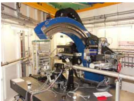
Fig. 8.4: Top: Specimen holder for radioactive samples. Bottom: Detector portal suited for (micro) x-ray beam experiments with radioactive samples.
