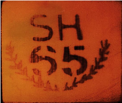
Figure 3: SNP crystal illuminated at low temperature. The illuminated areas are absorbing the visible light. We are using a crystal of 5 by 5 by 5 mm 3 .
