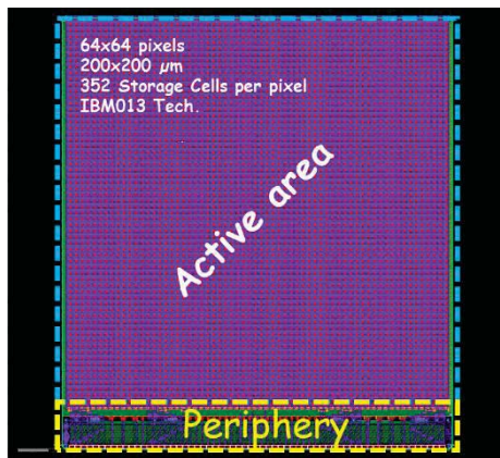
Figure 1 Layout of the AGIPD 1.0 single chip assembly. The active area and periphery (biasing blocks and command based interface) regions are marked.
