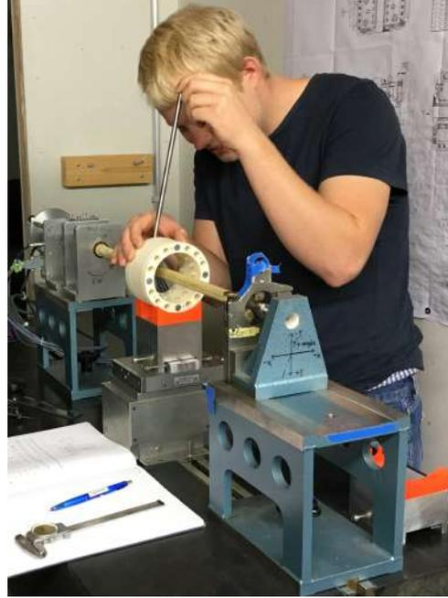
**Figure 24:** Image taken during the optimization of the magnetic field inside a Halbach ring. After each rotation of a magnet the field inside the ring was remeasured with the rotation coil (see Section 4.4).
