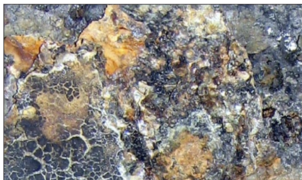
Figure 1: Macro-photograph of the inner surface of the corroded tank showing deposit layer (Sample 2)
