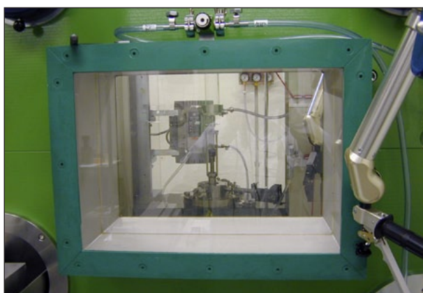
Figure 4: A remotely operated mechanical test machine, as seen behind its shielding.
