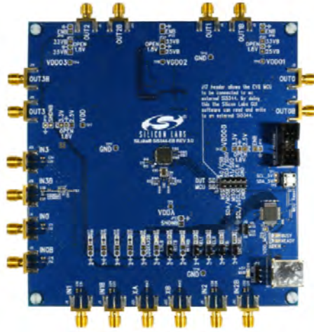
Figure 6.2: The Si5344 Evaluation Board. Central on the PCB the Si5344 is visible as well as the control MCU on the lower right side. Also, four in-and outputs as well as an external reference signal input XA/XB and a ten pin header for serial interface programming are visible. Adapted from [40].
