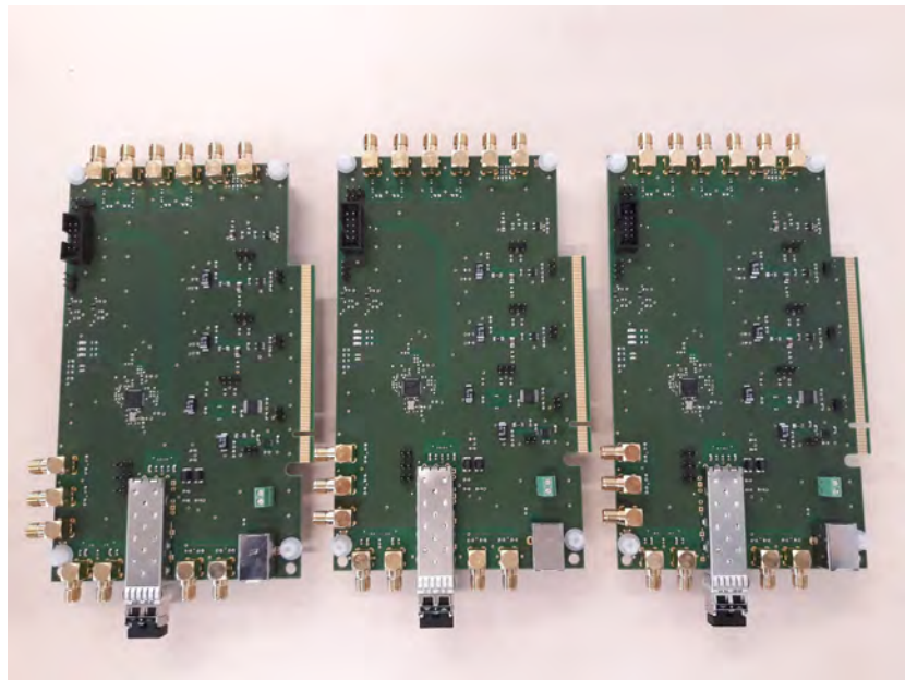
Figure 6.9: Three CTB prototypes. On the lower side of the picture the optical transceiver can be seen; the output side of the board can be observed at the top of the image.
