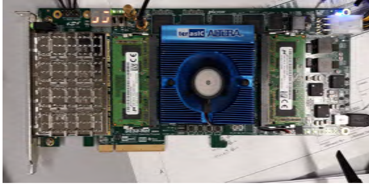
Figure 7.2: Arria 10 FPGA used as the SPI host for the CTB.
