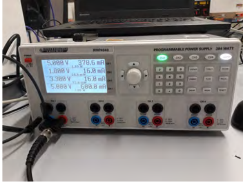
(a) The Rhode-Schwarz Hameg HMP4040 programmable power supply used for testing of the CTB.
