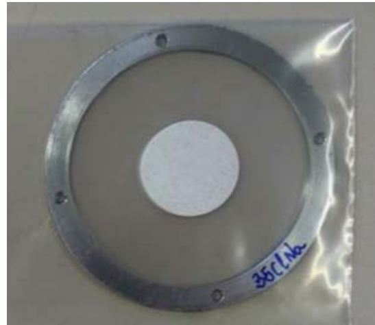
Fig. 2: Sample of \text{Na}^{35}\text{Cl} used in the experiment inside a Mylar bag.
