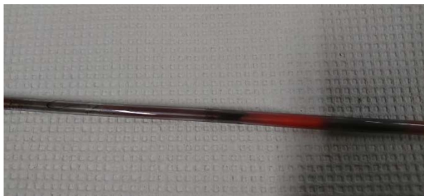
Fig. 3: Se coated quartz column after thermal conversion at 200 °C. Both red and grey areas are visible, indicating incomplete conversion.
