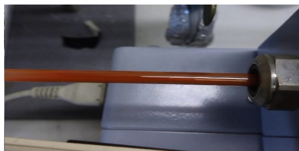
Fig. 2: Newly a-Se coated quartz tube, crimson red.
