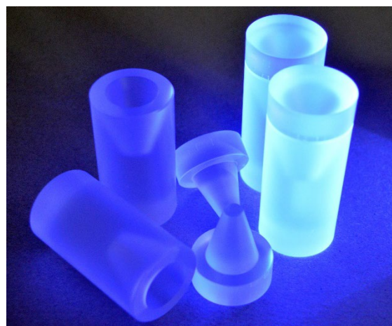
FIGURE 2: Plastic scintillator vials illuminated by UV light to stimulate emission of scintillation light.
