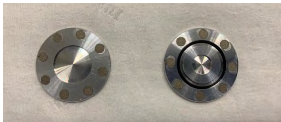
Figure 3: The coin target (24 mm diameter, 2 mm thick).
