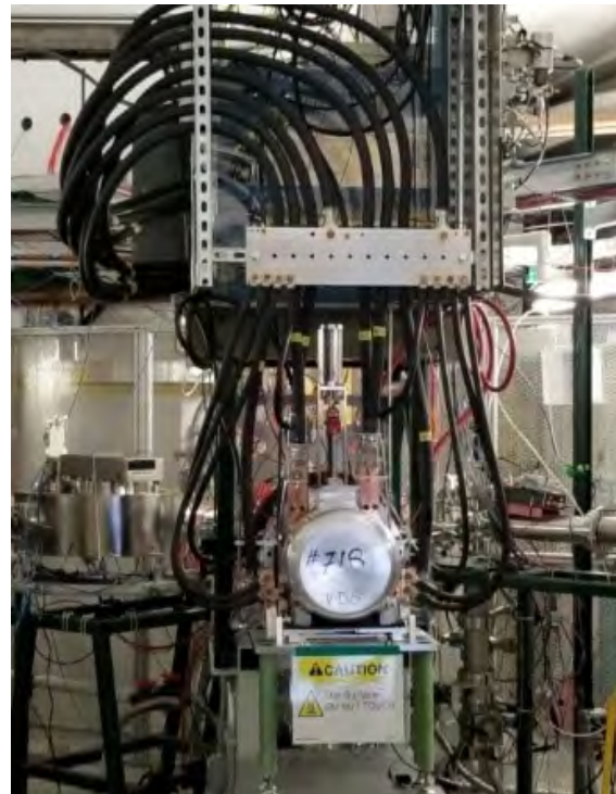
Figure 1: The BMIS system makes use of ISOLDE target modules coupled to front-end. Be-10 samples provided by PSI were loaded into the target container of the target modules to provide beams for reacceleration and use in nuclear science experiments.
