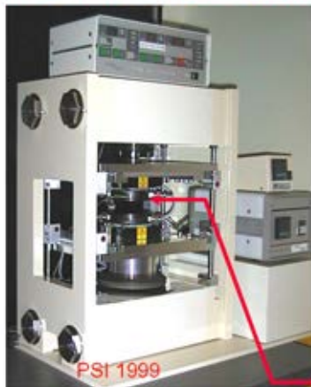
Figure 5.15: A simple (oil) hydraulic imprint machine.
