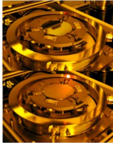
Figure 5.22: Jenoptik HEX03 nanoimprint machine with and integrated adapter for a Süss alignment fixture for an anodic bonder. Alignment is possible by using the appropriate mask aligner.
