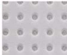
Figure 5.35: Example for etching as a pattern transfer process after NIL.
