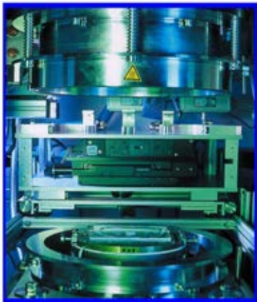
front side with opened embossing chamber and inserted microscope
