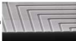
Figure 5.39: Example for electroplating as a pattern transfer process after NIL.
