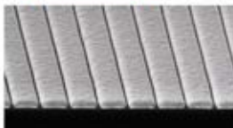
Figure 5.39: Example for electroplating as a pattern transfer process after NIL.
